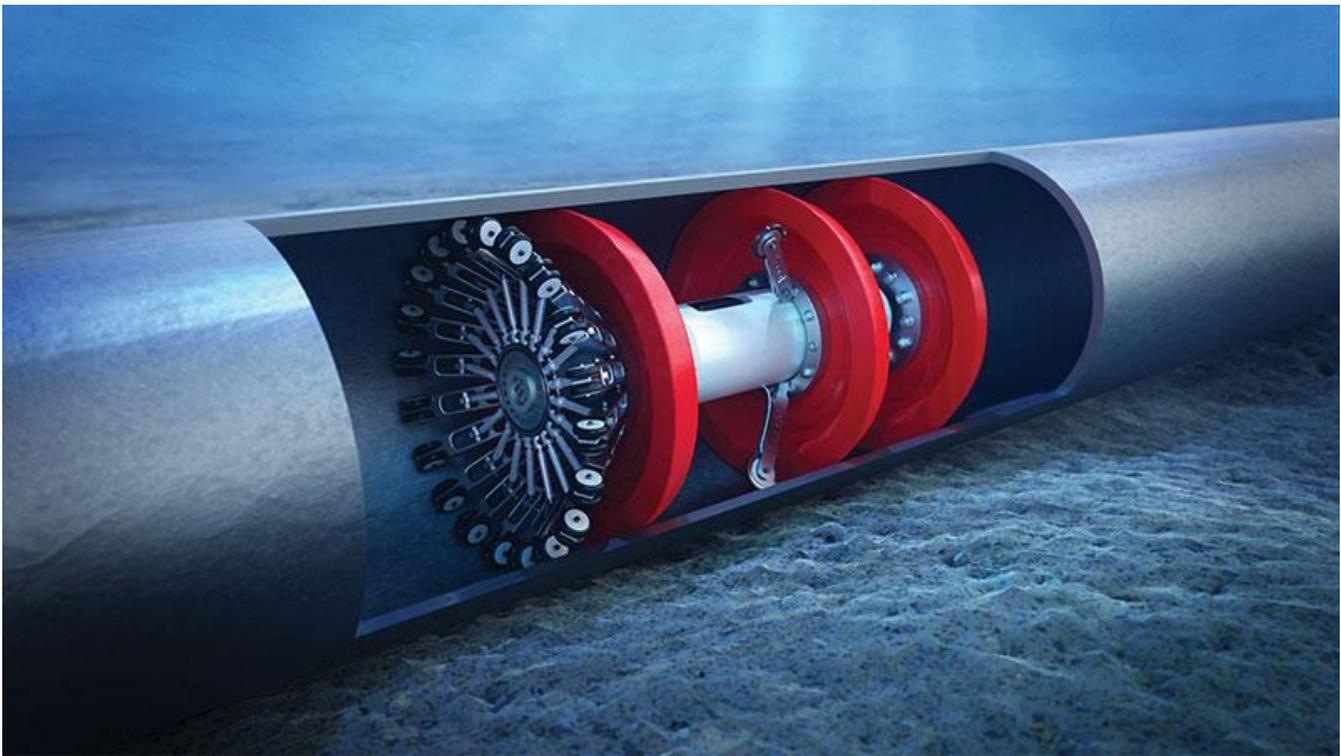
» Figure 5.7. Depiction of a typical smart pig in use in a pipeline.
